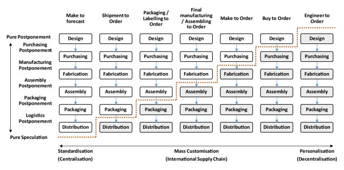
Fig. 10 Postponement strategies for different supply chain structures and logistics (adapted from [81])
