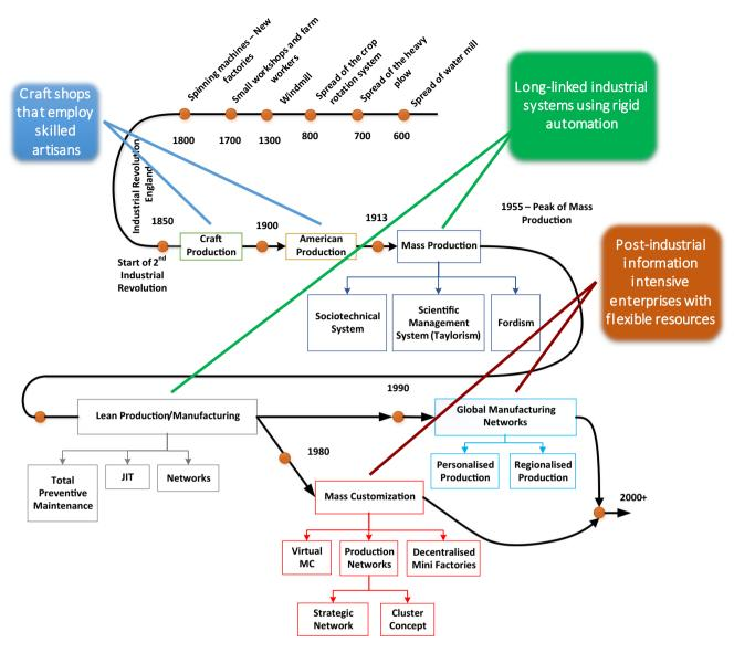
Fig. 2 Evolution of manufacturing paradigms (adapted from [11])
