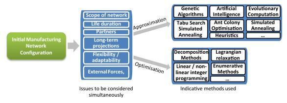
Fig. 8 Issues to be considered during the initial manufacturing network configuration and indicative methods used
