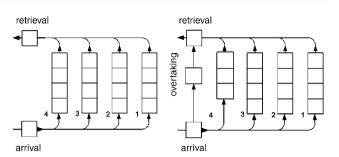
Fig. 6 Example of mixed-bank buffers with and without overtaking lane [14]
