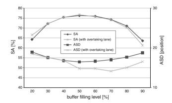
Fig. 8 Re-sequencing performance with variation of the buffer filling level [14]
