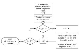
**Fig. 4** Algorithm for calculation of sequence violations by means of the sequence displacement [14]
