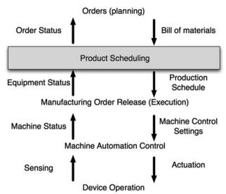
Fig. 2 The central position of product scheduling in the manufacturing control
