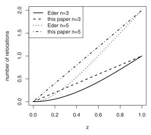
Figure 8: Comparison of two different models for the number of relocations  $\beta$  during a retrieval operation for multi-deep AS/RS (n = 3 and n = 5); Eder [23] and this paper.
