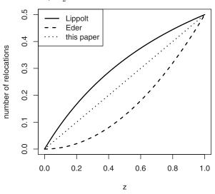
Figure 7: Comparison of three different models for the number of relocations  $\beta$  during a retrieval operation for double-deep AS/RS; Lippolt [10], Eder [23] and this paper.
