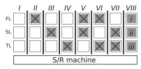
Figure 3: Triple-deep AS/RS. Storage good i shall be retrieved out of channel III.
