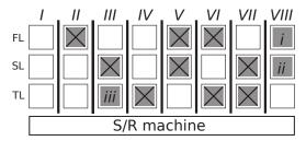
Figure 4: Triple-deep AS/RS after the first relocation.
