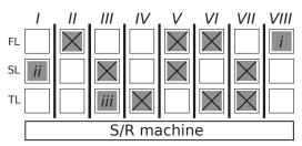
Figure 5: Triple-deep AS/RS after the second relocation.
