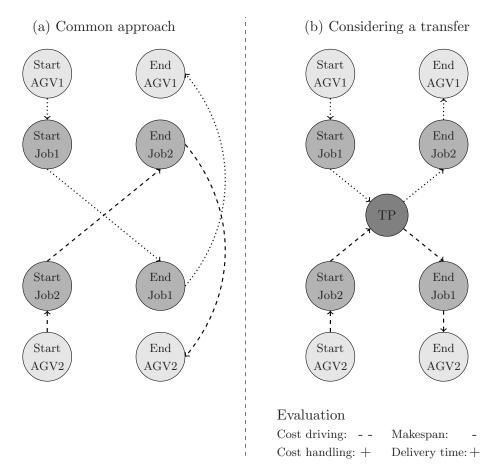
Figure 1: Comparison of a task assignment neglecting (left) and considering (rigth) a transport load transfer
