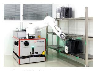
Figure 2: Multiple-load AGV equipped with a robot arm handling at a shelf in a semiconductor production facility (reference: www.fabmatics.com)
