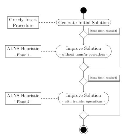
Figure 3: Optimization process: creating an initial schedule and applying the ALNS in two phases.
