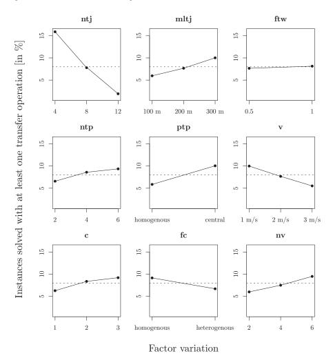
Figure 7: The influence of basic system characteristics to the percentage of solutions solved by transport load transfers
