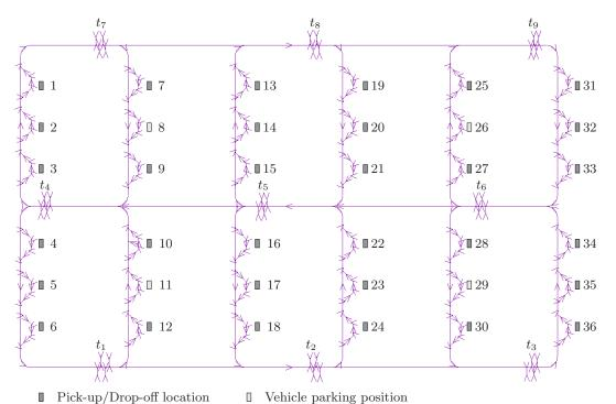
Figure 8: Layout of the simulation model with a dimension of 50 m in width and 30 m in heigth
